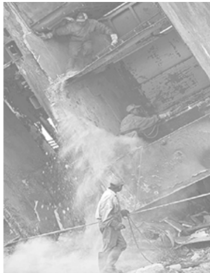
Fig. 9 The hatches and pockets of vessel may contain explosive or inflammable gases (Photo: Reichmann, 2005)
